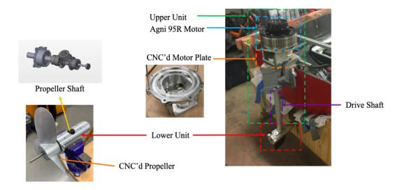
Figure 3: Diagram of manufactured components in new propulsion system
