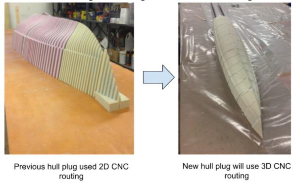
Figure 2: New process to CNC cross sections for male mold
