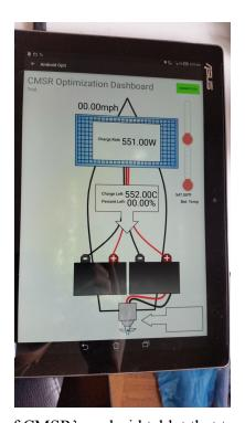
Figure 6: Dashboard of CMSR's android tablet that tracks data from sensors
