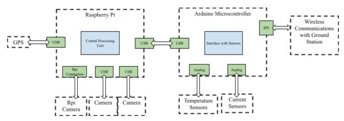
Figure 4: High-level schematic of our system of sensor readings with the Arduino as well as GPS and camera data processing by the Raspberry Pi.
