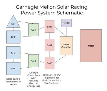
Figure 1: Overview electrical diagram of power system
