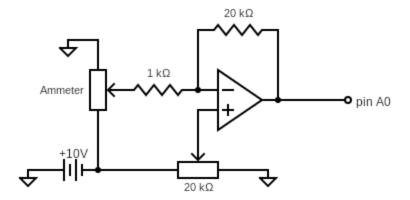
Figure 5: Testing diagram to measure low currents in system
